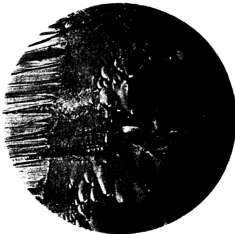
FIG. 9. Smectic structure of ethyl p -azoxybenzoate. From left to right: crystalline solid; pseudomorph of solid; smectic, focal conic structure; liquid state. From Lawrence (215).
